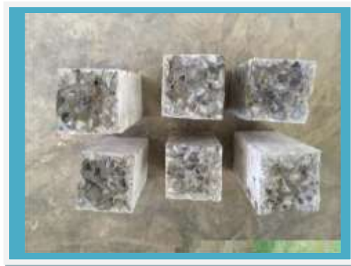
Figure 4. The condition of the beam specimen after splitting
