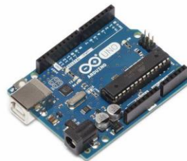
Figure 1. Arduino Uno R3
