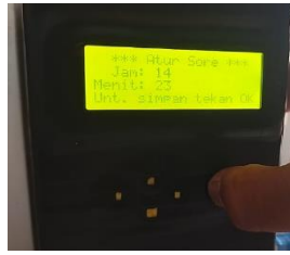
Figure 17. Tool to Dispense Fish Feed on Schedule
