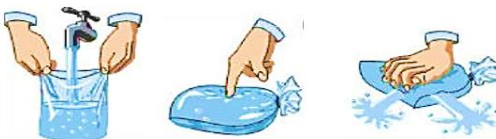
Figure 3. Experiment demonstrating hydrostatic pressure
